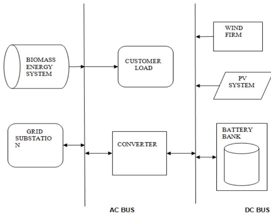
Figure 1. Parallel integrated power system
